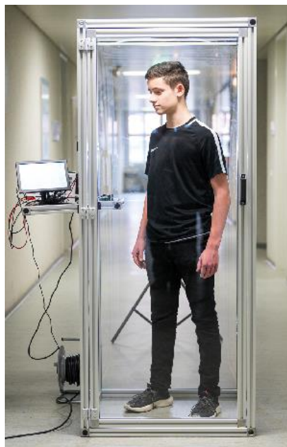
Fig. 5 Walk-in measurement chamber for the investigation of CO 2 and TVOC outgassing from humans.
