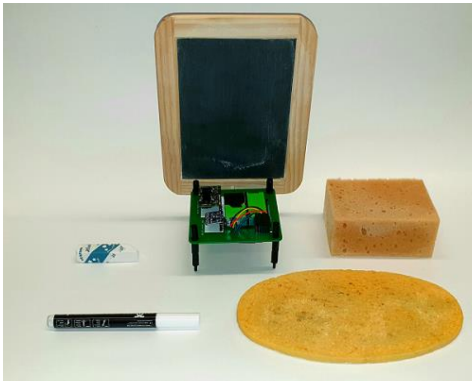
Fig. 7 Experimental setup for the investigation of particulate matter in chalk. The measuring board is snapped onto the lower edge of the panel.
