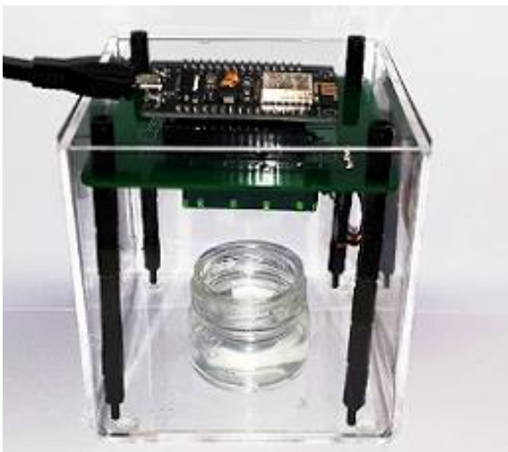
Fig. 3 Experimental setup for measuring the ethanol concentration of 5 solutions.
