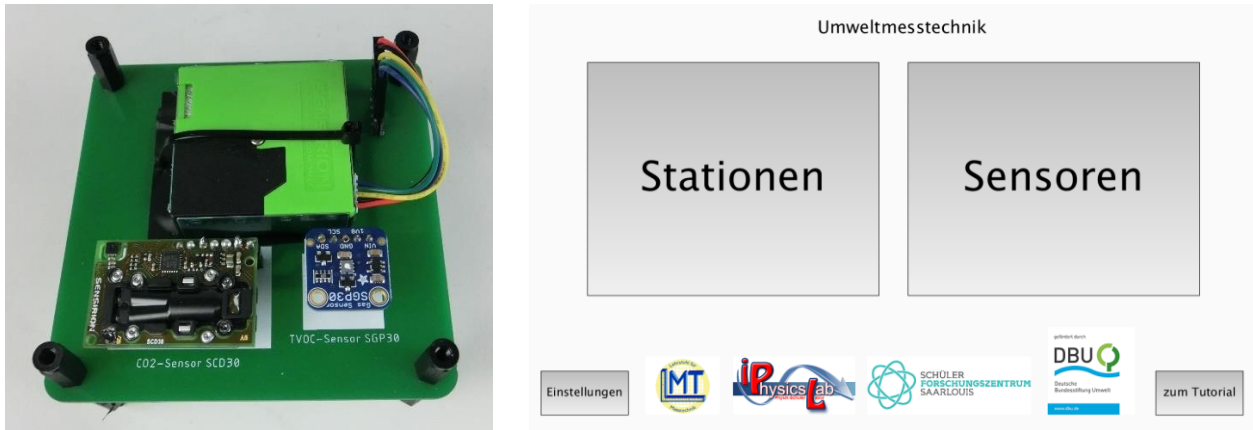
Fig. 1 Left: Measurement board with three sensor modules. Right: Main menu of the measuring software.
